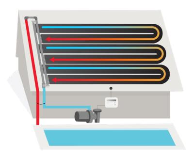
Thermal Solar Pool Heating is a simple and effective form of pool heating. Pool water is pumped through a series of tubes, known as a solar collector which is installed on your home, shed or other nearby building. The solar collector absorbs the sun's free heat and transfers it to the pool water that is being pumped through it. This heated water is then returned back to the pool.
